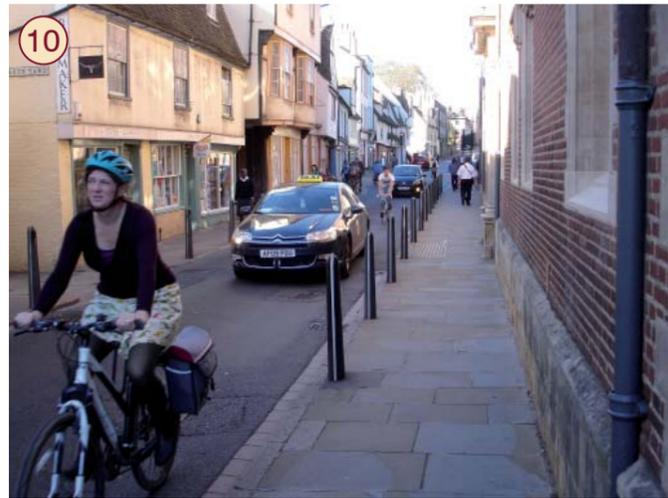
10 Carriageway narrowed to allow wider pavements outside shops and college. Reflective band designed into bollard
